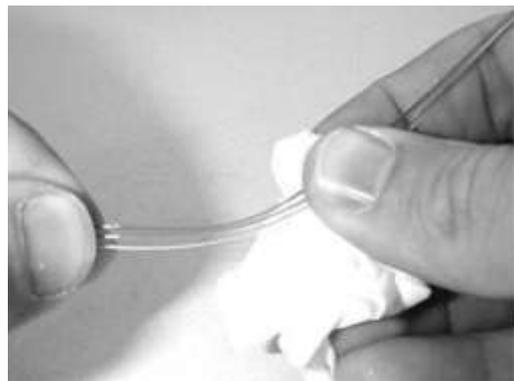
**Figure 8 – Clean the optical fibers.**
