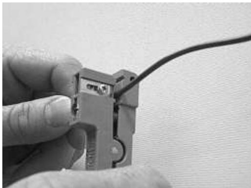
**Figure 7 – Ring cut the buffer tube.**
