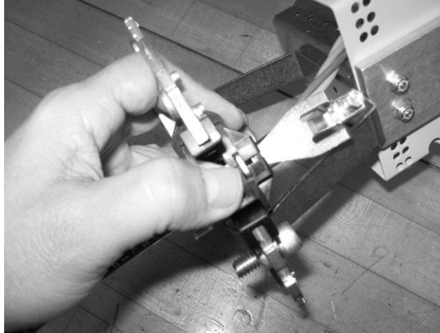
Figure 7 – Insert cable attachment bracket into the appropriate port of the metal frame.
