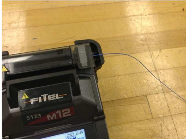
**Figure 4 – Place the splice and heat shrink sleeve in the heater.**
