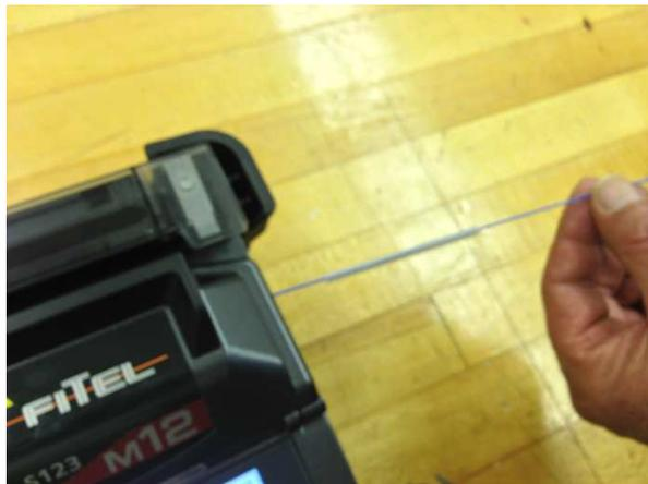
**Figure 3 – Slide the heat shrink over the splice.**
