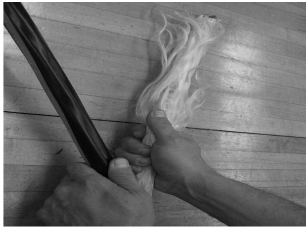
Figure 6 – Remove the outer jacket.
