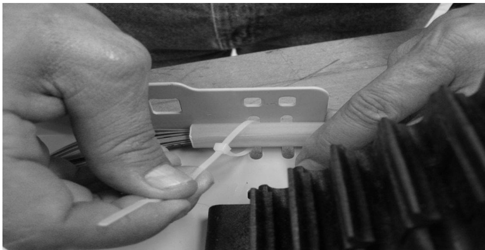
Figure 19 – Fasten transport tubes to storage basket.
