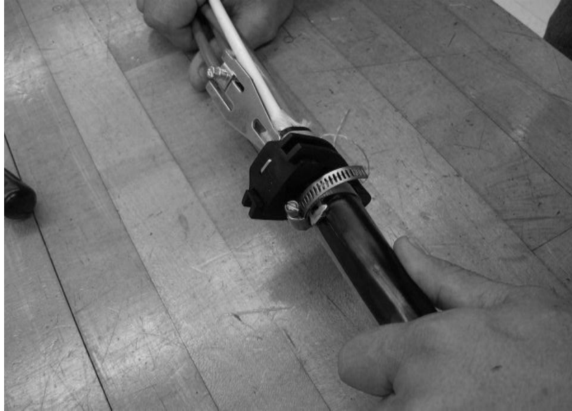
Figure 12 – Install hose clamp on cable attachment bracket.
