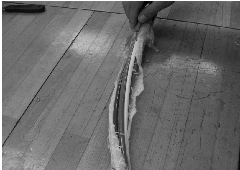
Figure 8 – Cut and remove binder thread
