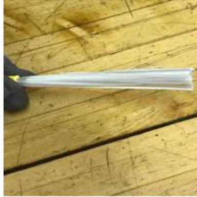
**3.6** Wrap the rip cord around the pliers and pull the rip cord through the outer jacket to the inner ring cut.
