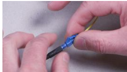
24. Unscrew the boot assembly from the housing.
