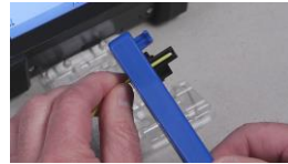
5. Ring cut and remove the outer jacket at 20mm.
