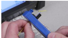
8. Ring cut and remove the outer jacket at 26mm.
