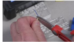
6. Remove the aramid yarn at 20mm.
