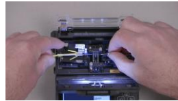
19. Remove the cord from the left cordage holder and release the ferrule from its ferrule holder on the right.
