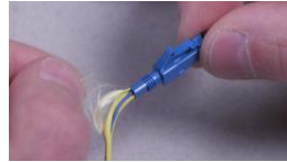
26. Pull out the outer jacket and aramid yarn from the tail of the housing.
