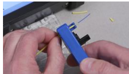
9. Split the outer jacket lengthways at 45mm.
