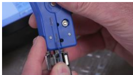
15. Use measuring line to ensure that exactly 7mm of 900µm coating protrudes from the extreme end of the holder.
