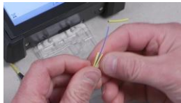
10. Fold the aramid yarn back, placing one half on each side of the cord.
