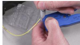
12. Mark the 900µm buffered fiber at 23mm. In case fiber is curved, mark on back side of the fiber.
