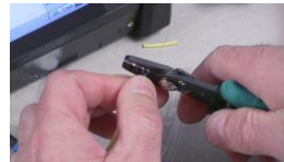
13. Remove the primary 900µm and secondary 250µm coating of the buffered fiber at 23mm.
