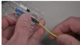
1. Insert the cord through the boot housing assembly and spring.
