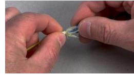
28. Spread the aramid yarn over the tail of the housing and hold the aramid yarn in place by sliding the clamp up to the housing.
