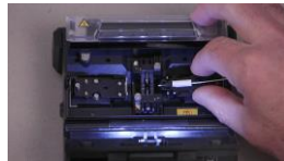
3. Load the ferrule holder onto the right carriage of the splicer.
