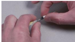
23. Slide the spring over the protection sleeve to the ferrule unit.
