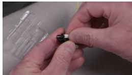
2. Load ferrule unit into the ferrule holder. Push forward, then push tip down.
