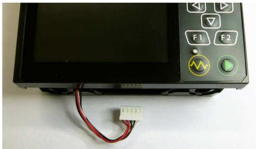
3. Remove the connector of battery.
