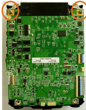
2. Remove all wiring connected to the electric board. And remove 2 screws which fix the board.
