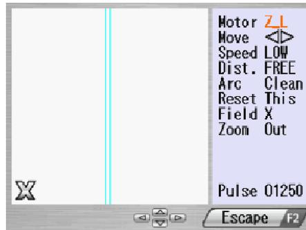
1. Select "Manual Splicing" in the Tool menu screen and press .
