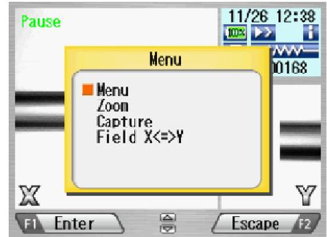
•If the fibers fail the inspections for cleave criteria, the fusion cycle is paused and an appropriate error message is displayed as below. Press **▼** to temporarily hide message and check the state of the fiber. Open the windshield, remove the fibers after READY is displayed and retry the splice by repeating the entire procedure, starting from the fiber preparation process. To ignore the error and continue the cycle, press **OK** and press **Enter**.
