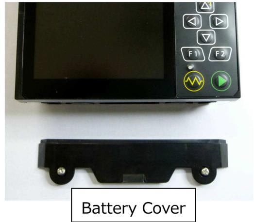
2. Remove the 2 screws of battery cover, and remove it.
