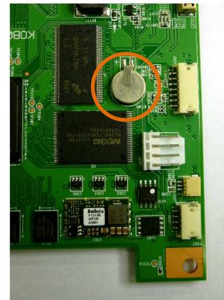
3. There is a built-in battery in the back of the board. Please cut the fitting off and tear the battery away.
