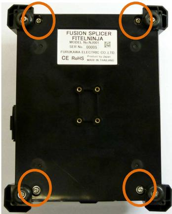
1. Remove the 4 screws, and remove the bottom case.
