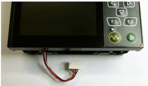
3. Remove the connector of battery.
