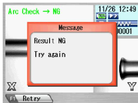
5. If result is NG, repeat the arc check until the new values are acceptable. It is necessary to remove the fibers and prepare them again with a new cleave. If unsatisfactory results are obtained after 4 arc check attempts, inspect the electrodes for wear or damage, and replace them if necessary.
