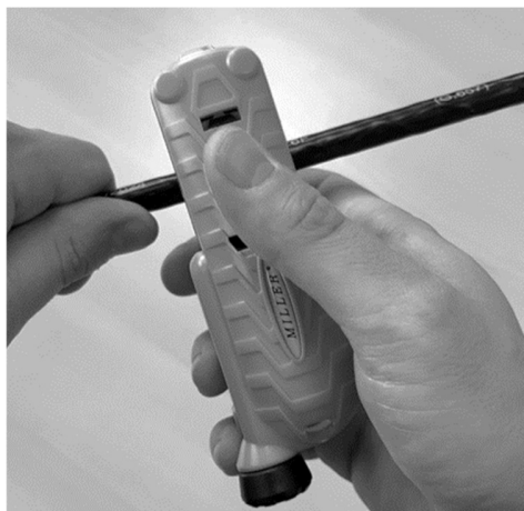
Figure 24 - Ring cut the outer cable sheath
