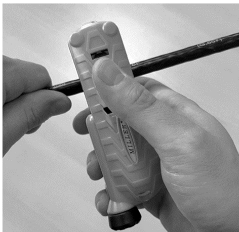
Figure 17 . Ring cut the cable sheath
