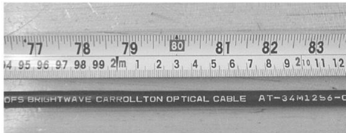
Figure 23 - Measure and mark the mid-span sheath opening
