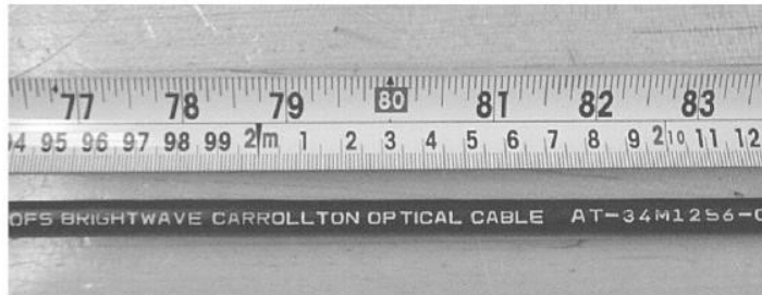
Figure 16 - Measure and mark the cable.
