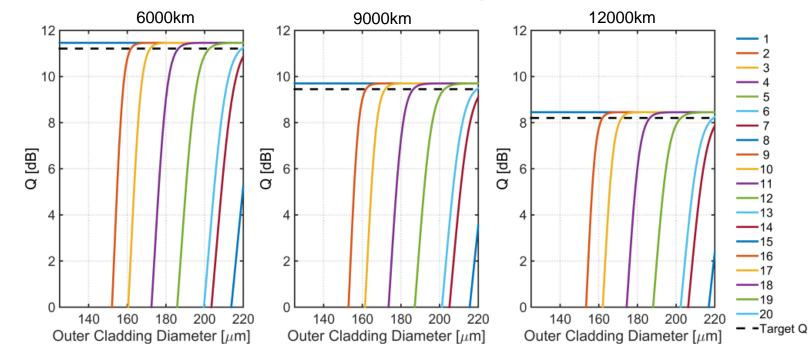
• At 6000km, with 6 cores, Q is 11dB worse at  $200\mu m$  OCD but no degradation at  $220\mu m$
