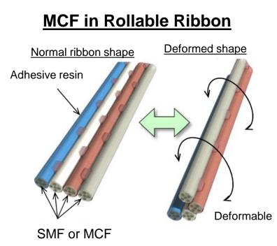
4-core MCF in Rollable Ribbon Achieved cabled density of 8.4 cores/mm<sup>2</sup>
