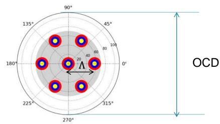
• Crosstalk between two trench-assisted cores:
