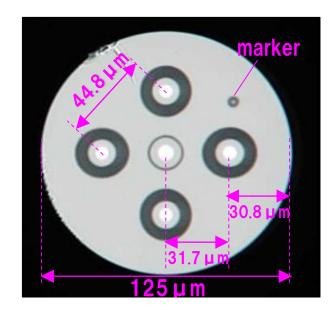
5-core, 125mm clad trench-assisted design G.657.A1 cutoff, MFD, bend loss Low crosstalk @ 1km length
