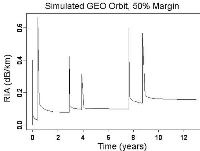
**Figure 3.** Radiation induced attenuation at 1550 nm versus time in a geosynchronous orbit. Flares were simulated assuming 4 major flares per decade with a total exposure of 60 krad (50% more than assumed from standard exposure with 20 mm Al shielding in a GEO [5]).
