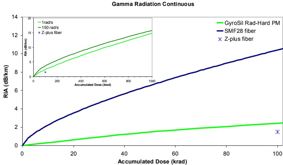
**Figure 2.** Radiation induced attenuation at 1550 nm versus accumulated dose of gamma radiation at a dose rate of 1 rad/s. The GyroSil Rad-Hard is compared with SMF28® [3] and the pure silica core Z-fiber® [4]. Inset shows the RIA at 1 rad/s and 150 rad/s dose rates up to an accumulated dose of 1 Mrad.
