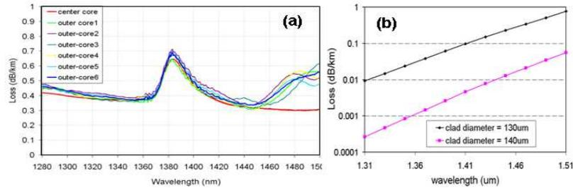
Fig. 1. (a) Measured attenuation spectra of 7-core MCF, (b) Calculated tunneling loss versus wavelength for clad diameter of 130 $\mu\text{m}$  and 140 $\mu\text{m}$ . This tunneling loss introduces an excess attenuation in the outer cores above that in the center core.
