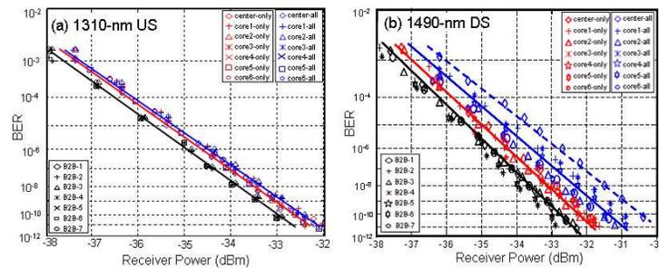
Fig. 6. BER performance for 1310nm US (a) and 1490nm DS (b) for all 7-core parallel transmission with 1:64 splitter for three cases: back-to-back (B2B, black), one core transmits only (core#-only, red) and all cores operate through the MCF simultaneously (core#-all, blue).
