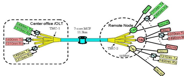
Fig. 5. Schematic diagram of a PON system using a 7-core MCF and two TMCs, 1310nm and 1490 nm DFB diodes as transmitters, APD as receivers.
