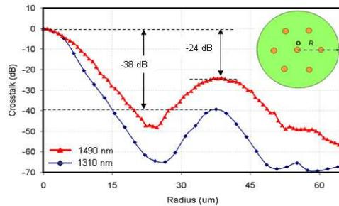
Fig. 2. Examples of the relative power versus the radius for crosstalk measurements.
