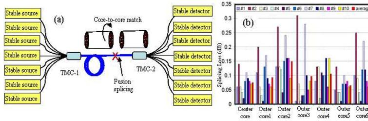
Fig. 4. (a) experiment set-up for study the splicing property of MCF, (b) splice losses of each core of seven-core MCF using PM fusion splicer.
