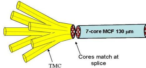
Fig. 3. Schematic diagram of tapered multicore fiber connectors.
