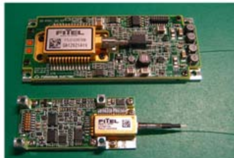
Figure 1: Conventional (top) and micro ITLA (bottom) comparison
